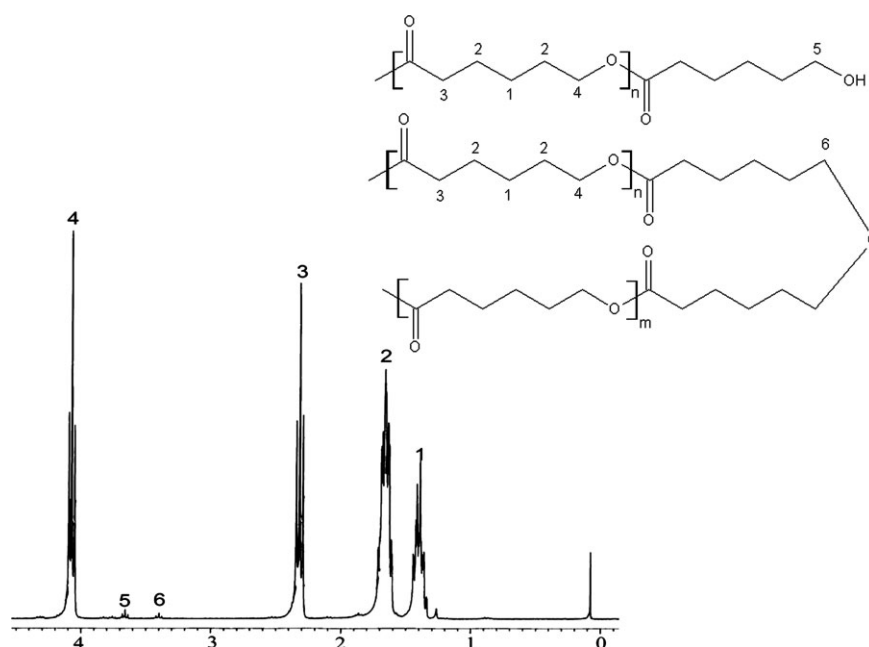
Figure 5 ^1\text{H-NMR} spectrum of the PCL prepared using neat \text{BF}_3 catalyst. The polymerization temperature was 110^\circ\text{C} ; polymerization time was 1 h. The \text{BF}_3 concentration was 75 ppm (vol) in the reaction mixture.
